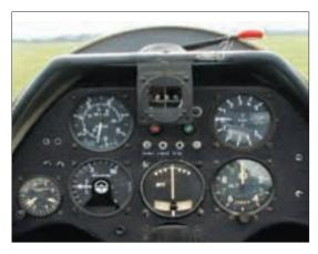
The instrument panel of a typical training glider in this case a K21, (clockwise from top left). Air speed indicator (ASI) - Compass - Vario (mechanical) - Altimeter - Turn and Slip indicator - Vario (electric) - G-meter.
